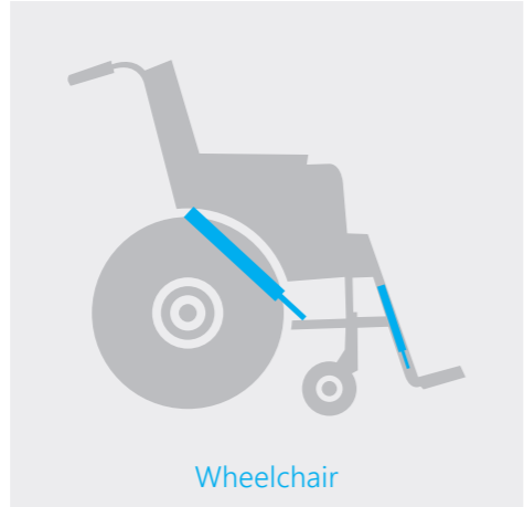
Lockable gas spring and Mechanical locking spring for adjusting the footrests and for the stand-up aid
