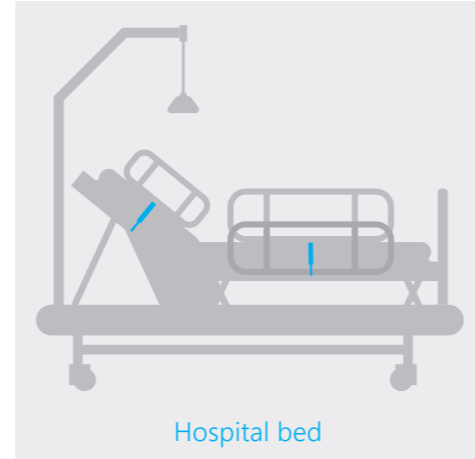
Rotary damper and Hydraulic damper for a comfortable and vibration-free adjustment of the swivelling bed side rails
