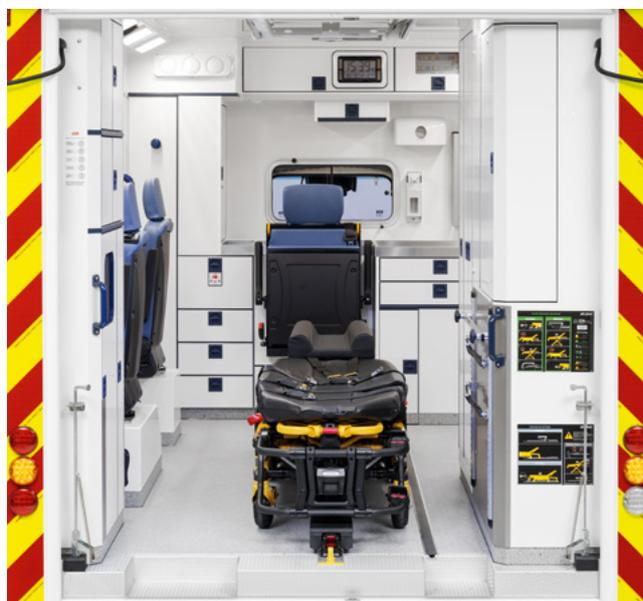
An airline track system is integrated into the floor for the loading of medical equipment and gear.
