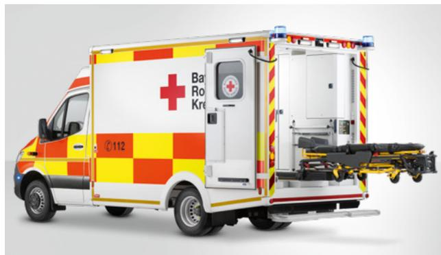
The Stryker Powerload stretcher system incl. the Power Pro XT stretcher facilitates the loading and unloading of heavy patients.
