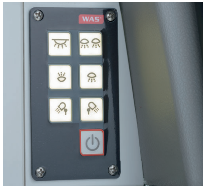
The efficient LED lighting system is also controlled from a panel at the rear cabinet.
