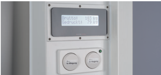
An electronic balance with tare functions to determine the exact weight of the patient; the appropriate weight note is created and printed.
