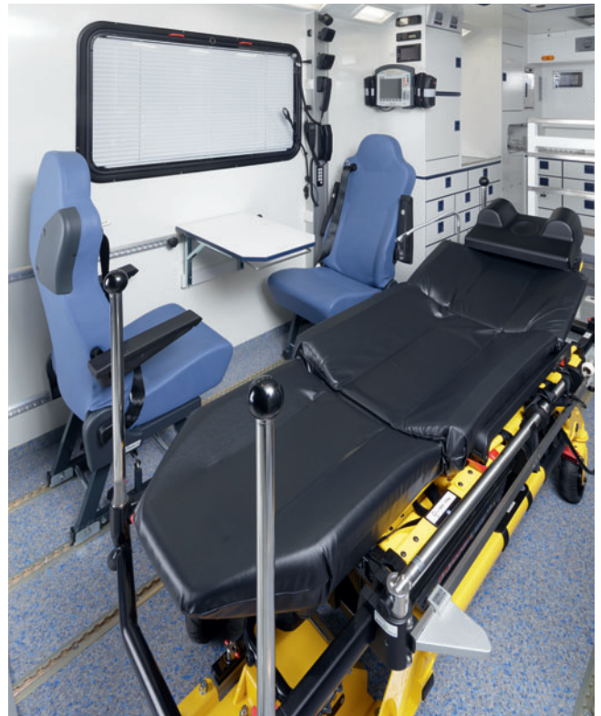
Attendants seats fixed on airline rails and working tables for a maximum of flexibility and comfort.
