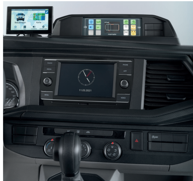
The central operating panel for warning lights is placed in a console mounted on the dashboard.
