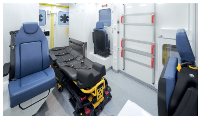
Multifunctional patient room with 3 seats left, right and at the head of the patient.
