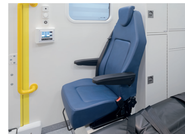
Comfortable seat with integrated three-point belt, 2 arm rests and adjustable back and head rests.
