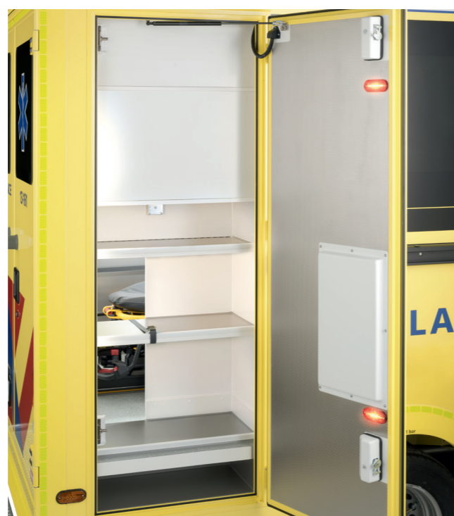
Space saving and easily accessible: emergency bags and other medical equipment in the large compartment.
